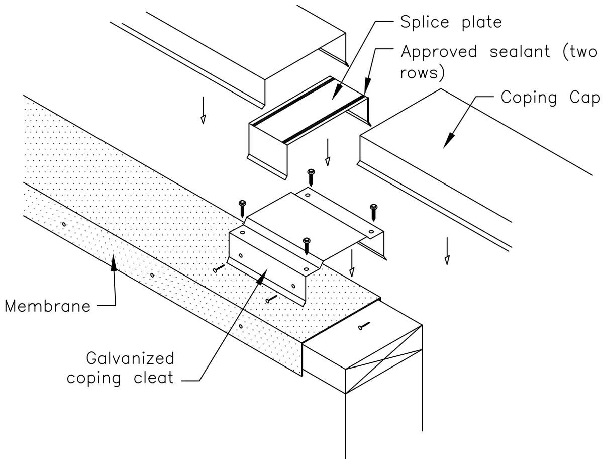
Note 1: Install the coping cleat using four hex-head screws with neoprene washers. Face nail the cleat using two roofing nails.
