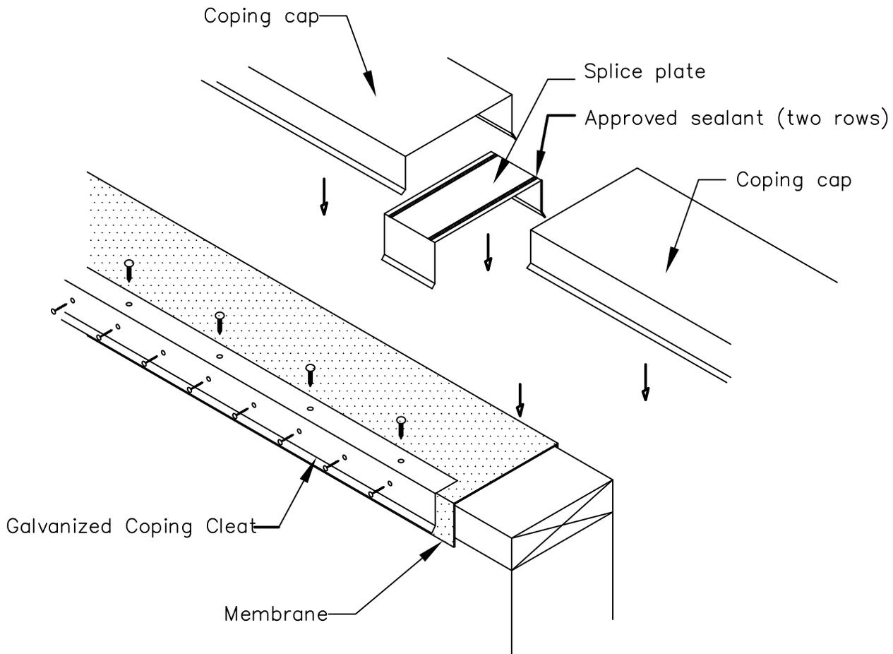
Note 1: Install the Coping Cleat using 1 ½-inch fasteners 12-inches on center. Face nail the Cleat using 1 ½-inch fasteners 12-inches on center.
