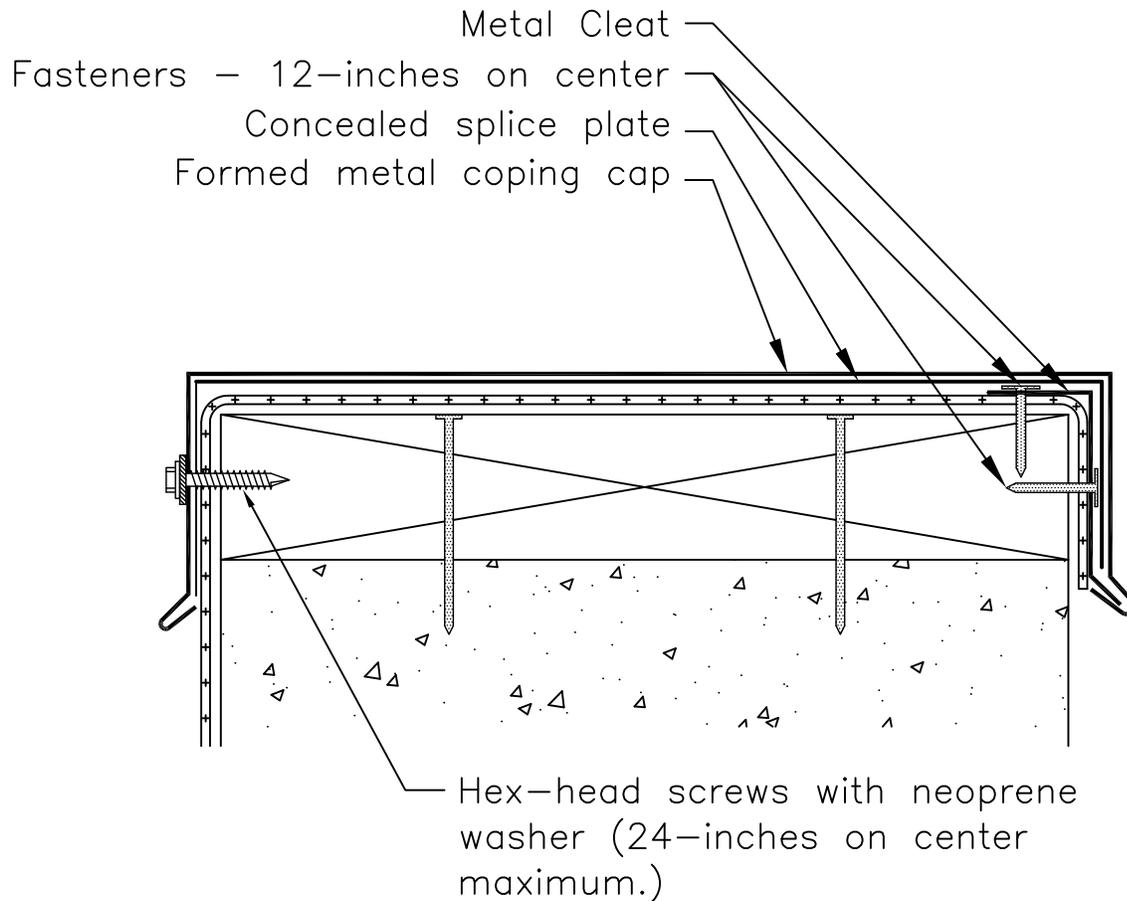
Note 1: All coping cap joints must utilize a 6-inch concealed splice plate.
