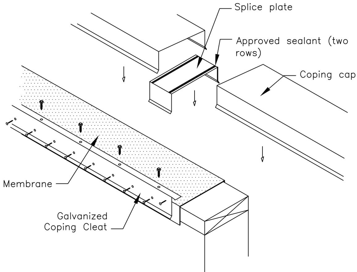
Note 1: Install the Coping Cleat using 1 ½-inch hex-head screws with neoprene washer 12-inches on center. Face nail the Cleat using 1 ½-inch fasteners 12-inches on center.
