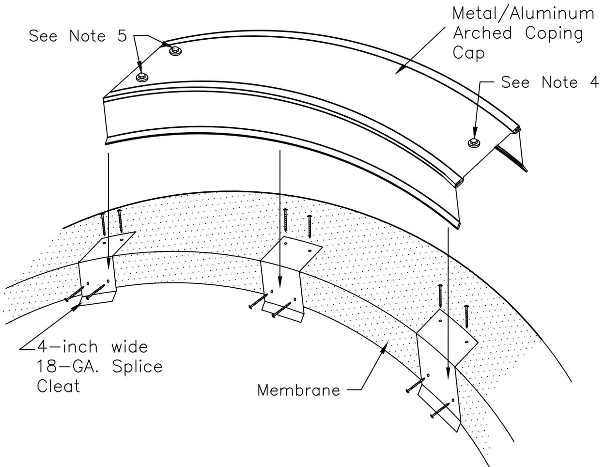
Note 1: Install 4-inch wide Splice Cleats 24-inch on center using four approved fasteners (must position a cleat at each joint).
