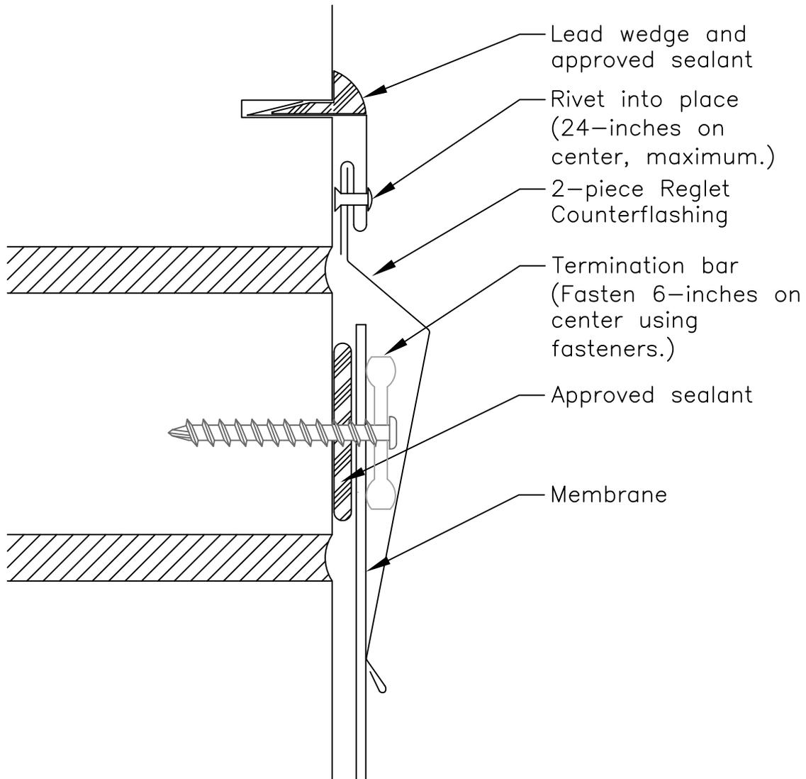
Note 1: This detail is only applicable to concrete or block walls.
