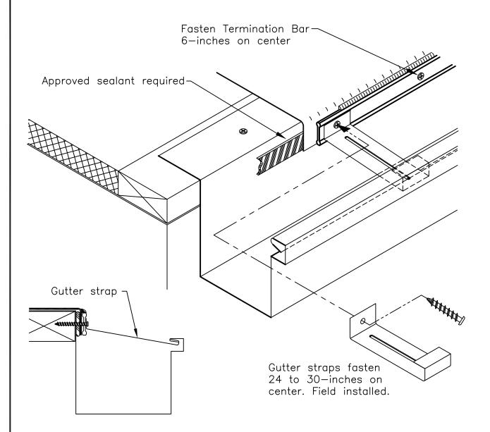
Note 1: A  $\frac{1}{4}$ -inch gap is required between sections of Termination Bar.
