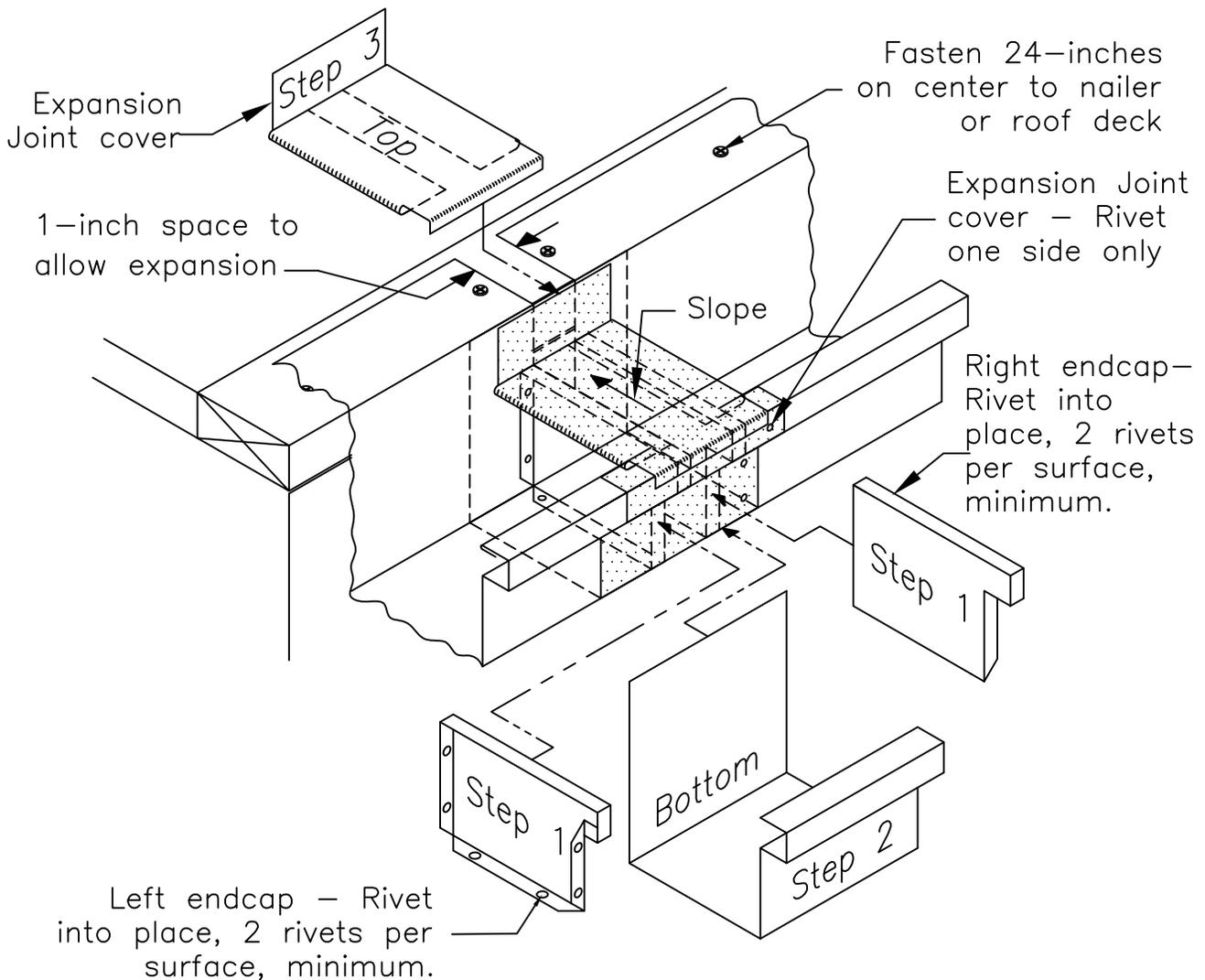
NOTE 1: Endcaps are to be riveted into position. On Expansion Joint cover rivet one side of the joint only.
