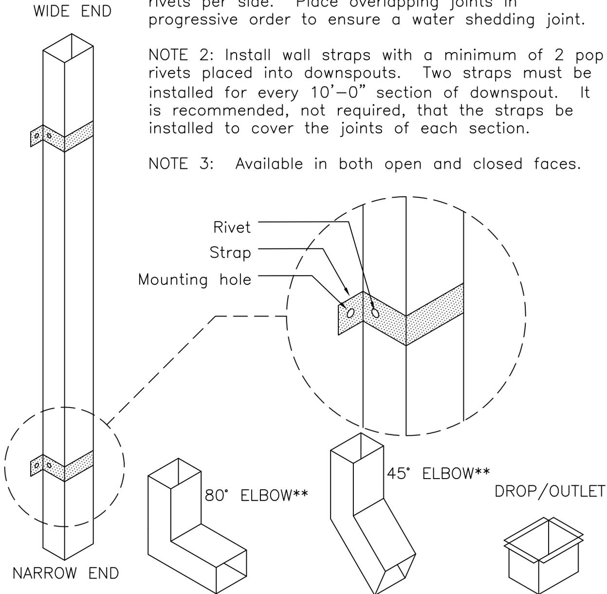
\*\* "A" & "B" Style elbows are available. "A" style elbows direct water away from the building. "B" style elbows direct water alongside the building.
