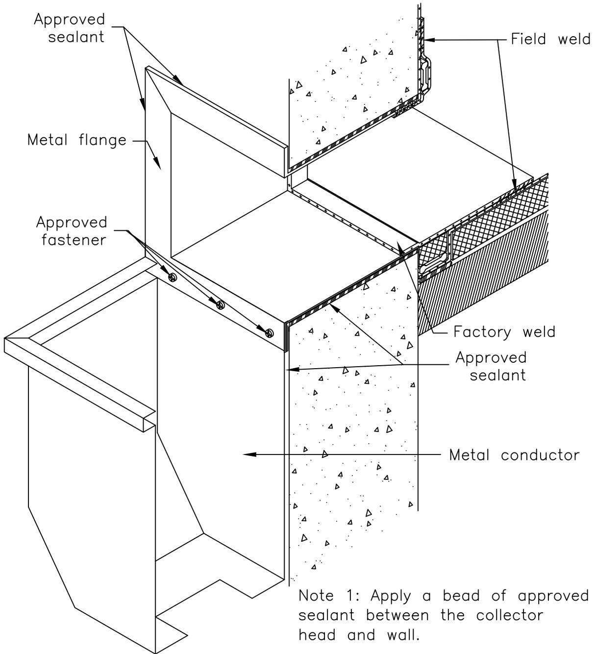
Note 1: Apply a bead of approved sealant between the collector head and wall.
