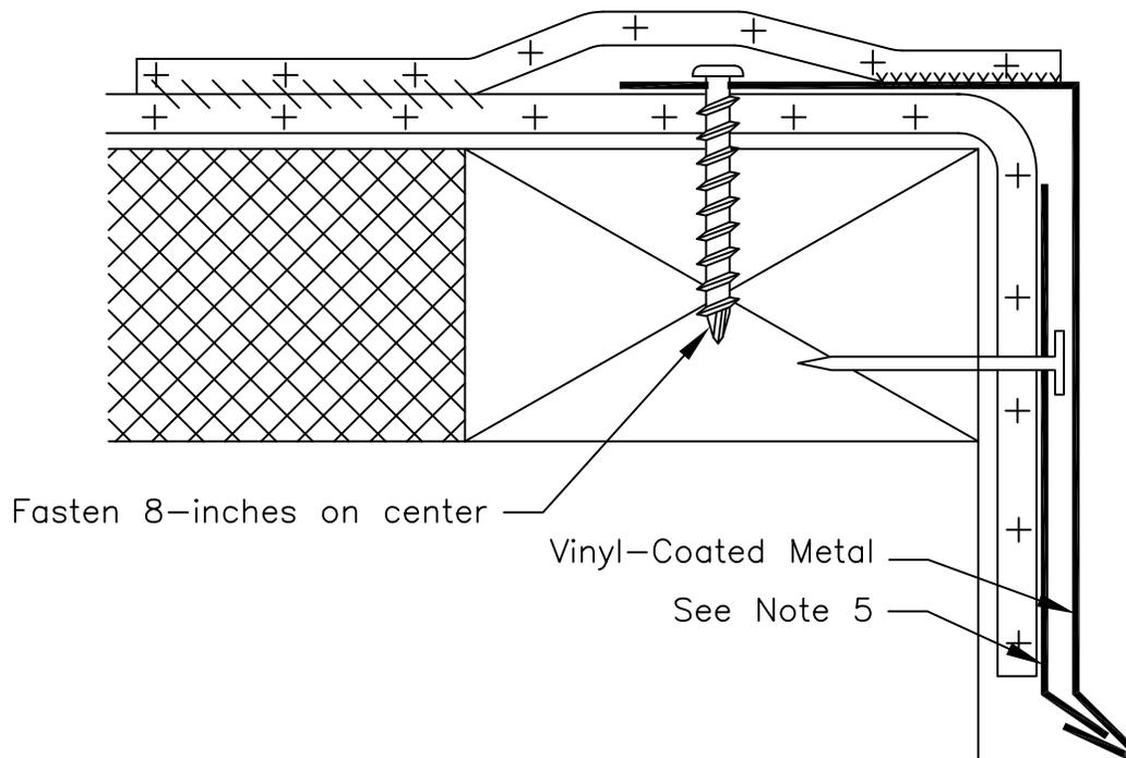
Note 1: Do not use this detail for fully adhered applications unless the membrane is back sealed using caulk or strip mastic.
