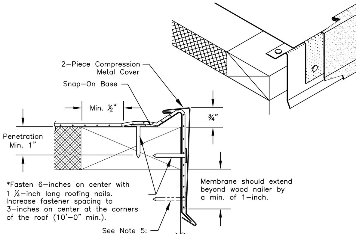
Note 1: The use of this detail is not to exceed a 2-inch per 12-inch slope.
