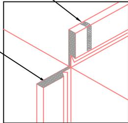
FIELD CUT PANEL RIBS AND BEND PAN OVER AT TRANSITION.
