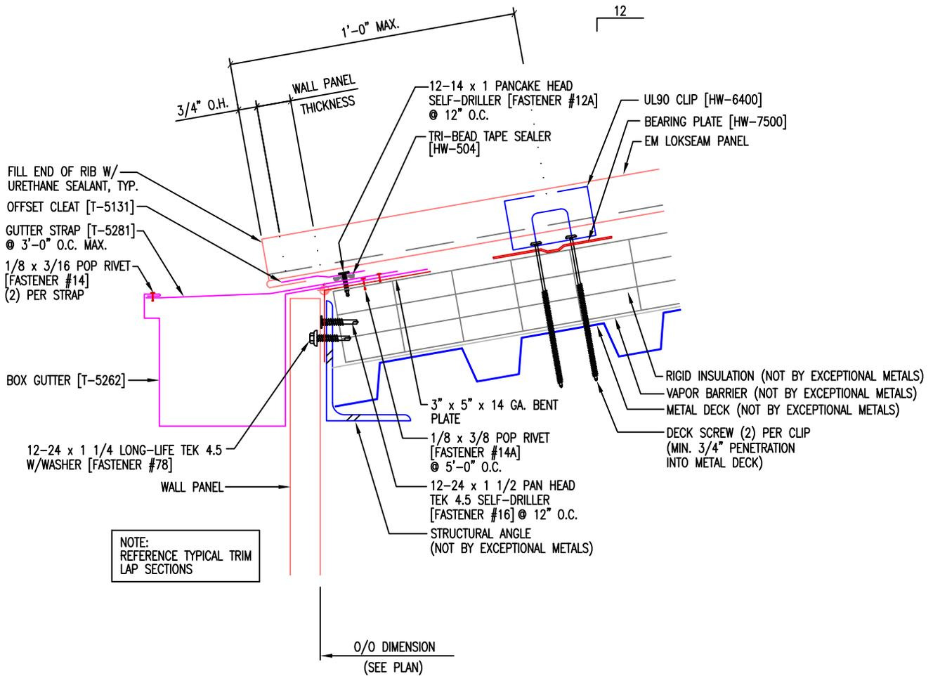
FIELD CUT PANEL RIBS AND BEND PAN OVER TO FORM OPEN HEM
