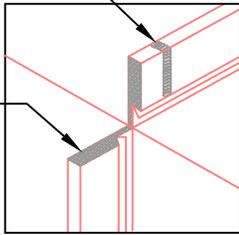
FIELD CUT PANEL RIBS AND BEND PAN OVER AT TRANSITION.
