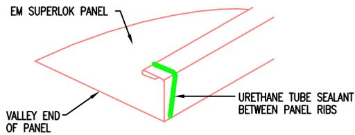
URETHANE SEALANT MUST COME IN CONTACT WITH TAPE SEALER TO FORM A WEATHERTIGHT SEAL
