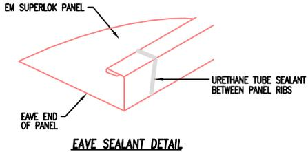
URETHANE SEALANT MUST COME IN CONTACT WITH TAPE SEALER TO FORM A WEATHERTIGHT SEAL
