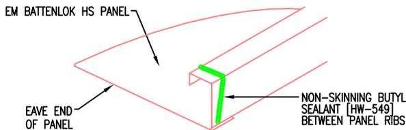
BUTYL SEALANT MUST COME IN CONTACT WITH THE DRIP EDGE TO FORM A WEATHERTIGHT SEAL
