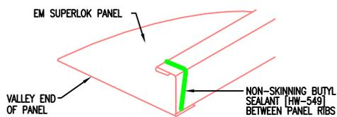
BUTYL SEALANT MUST COME IN CONTACT WITH THE OFFSET CLEAT TO FORM A WEATHERTIGHT SEAL
