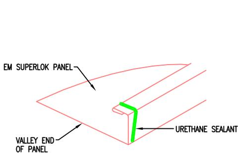
URETHANE SEALANT MUST COME IN CONTACT WITH TAPE SEALER TO FORM A WEATHERTIGHT SEAL
