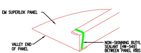
BUTYL SEALANT MUST COME IN CONTACT WITH THE OFFSET CLEAT TO FORM A WEATHERTIGHT SEAL
