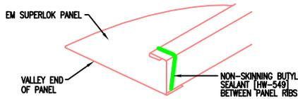
BUTYL SEALANT MUST COME IN CONTACT WITH THE OFFSET CLEAT TO FORM A WEATHERTIGHT SEAL
