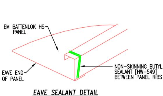
BUTYL SEALANT MUST COME IN CONTACT WITH THE DRIP EDGE TO FORM A WEATHERTIGHT SEAL
