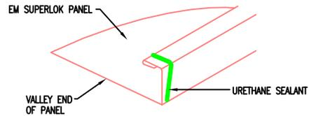
URETHANE SEALANT MUST COME IN CONTACT WITH TAPE SEALER TO FORM A WEATHERTIGHT SEAL
