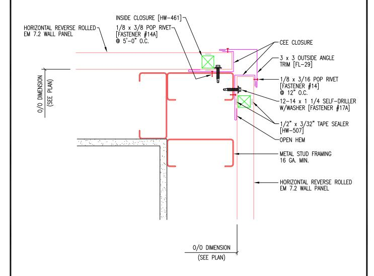
NOTE: EXCEPTIONAL METALS RECOMMENDS THAT A REVERSE ROLLED EM 7.2 PANEL BE USED IN HORIZONTAL APPLICATIONS SO THAT THE LAP FASTENERS CAN BE INSTALLED IN THE LOW RIBS.
