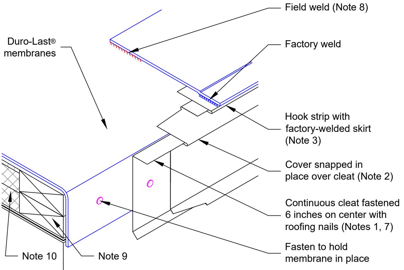
Note 1: A 1/8-inch gap is required between sections of cleat.
