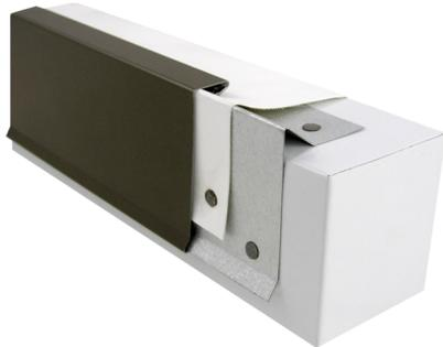
The 2-Piece Snap-On Compression system may be used as a perimeter flashing for single-ply roofing systems. The system consists of a 24-gauge Galvalume® base and a snap-on metal cover.
