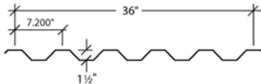
**EM PBA Panel:** The EM PBA panel can be used for wall applications and is striated as a standard, providing a unique design feature. The inverted ribs of the EM PBA panel provides for a discreet location of the exposed fasteners.
